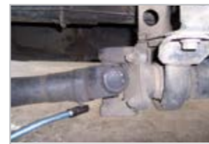
Right angled coupler used for greasing the axle of a low height truck where access to the grease fittings is only through a side
