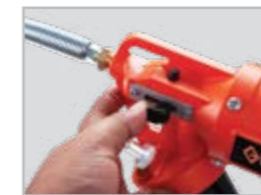
Slide backwards for Continuous Mode
