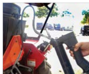
No twisting or kinking of hose
