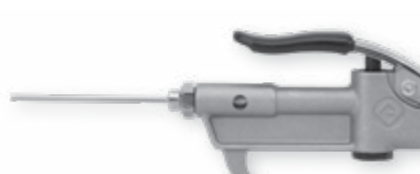
TYPE: N2 SS needle 2-15/32" (62 mm) long x 0.095" (2.4 mm) dia.
